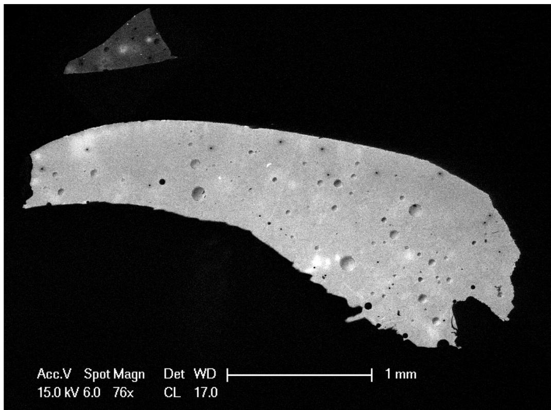
Figure 5: An image of Quartz glass 5a (top left) and 5 (centre) taken in CL on the SEM , EMMAC – University of Edinburgh. The lighter flecks are Fe, and not Ti that hasn't homogenised throughout the gel.
