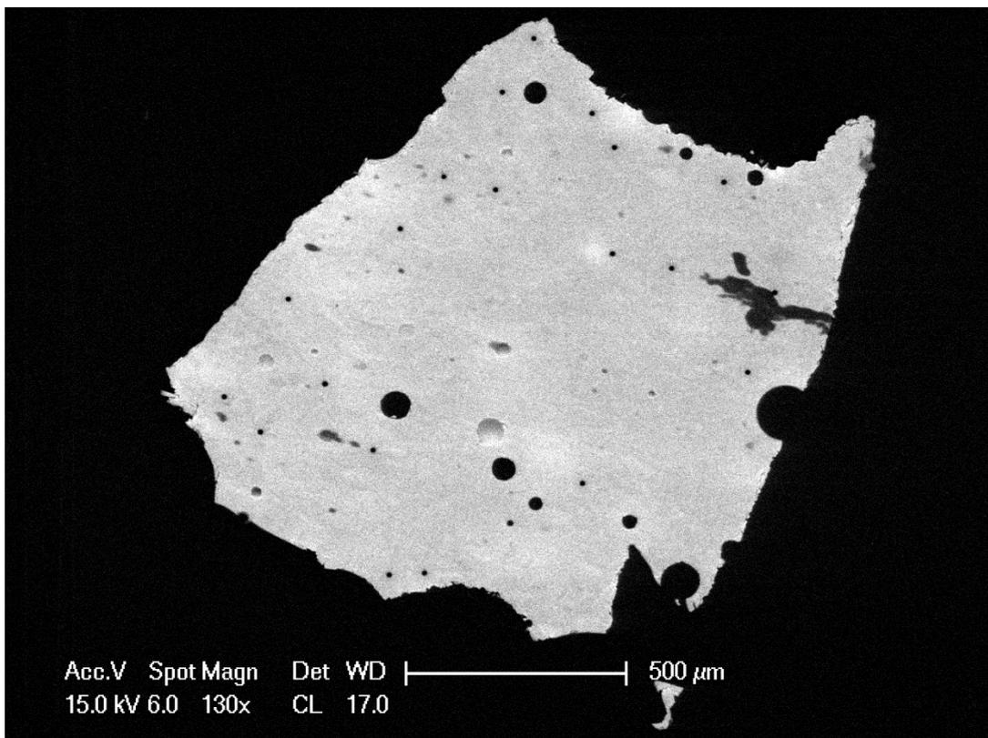
Figure 7: An image of Quartz glass 9 taken in CL on the SEM , EMMAC – University of Edinburgh. The lighter flecks are Fe, and not Ti that hasn't homogenised throughout the gel.
