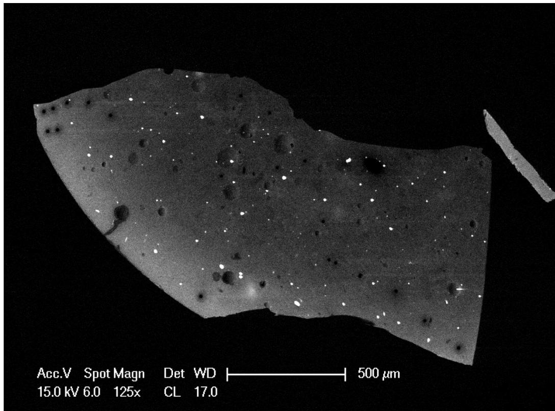
Figure 9: An image of Quartz glass 10 taken in CL on the SEM , EMMAC – University of Edinburgh. The lighter flecks are Fe, and not Ti that hasn't homogenised throughout the gel.
