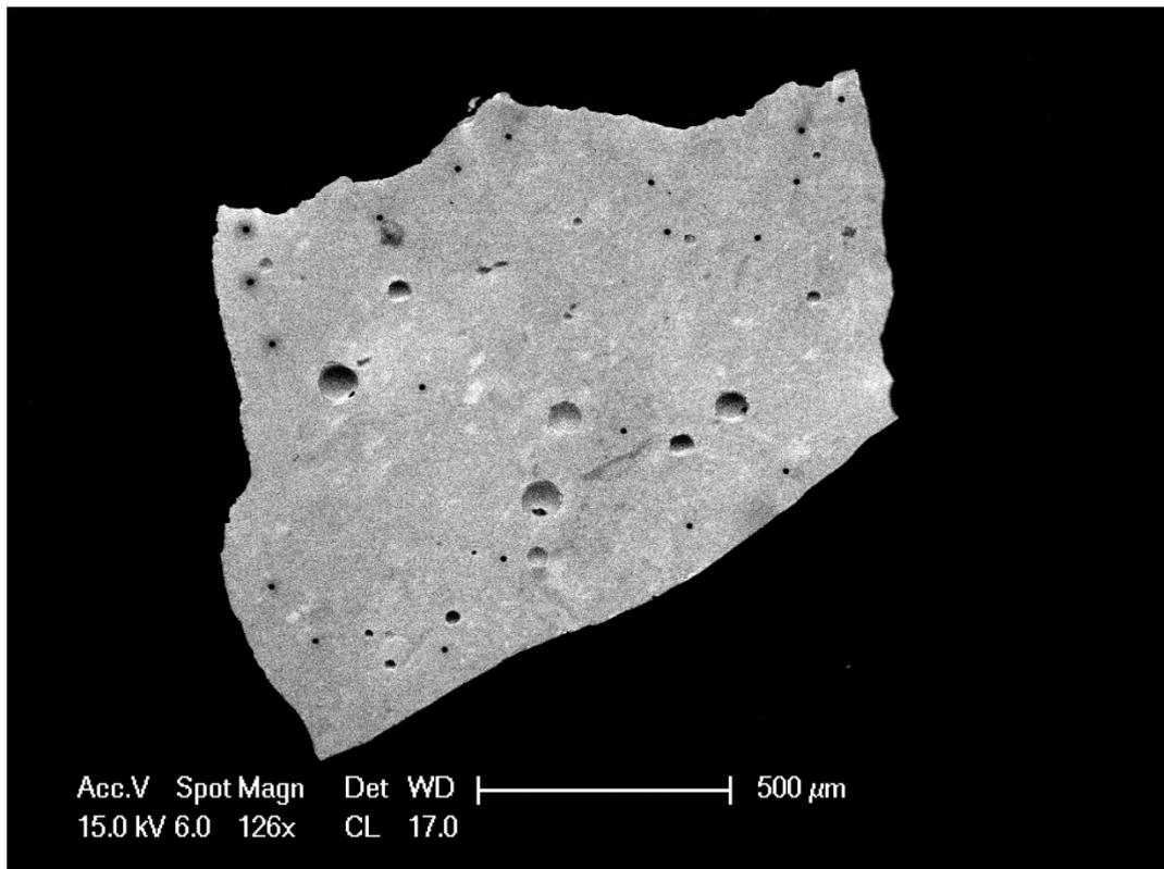
Figure 4: An image of Quartz glass 1 taken in CL on the SEM , EMMAC – University of Edinburgh. The lighter flecks are Fe, and not Ti that hasn't homogenised throughout the gel.
