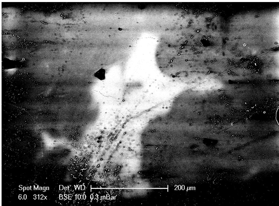
Figure 11: An image of FE brighter patch in one of the glasses, at the highest magnification ,taken in CL on the SEM, EMMAC – University of Edinburgh.
