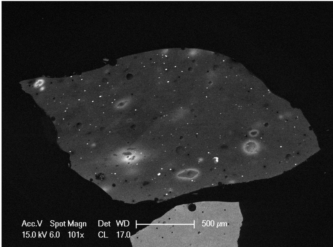
Figure 8: An image of Quartz glass 7 taken in CL on the SEM , EMMAC – University of Edinburgh. The lighter flecks are Fe, and not Ti that hasn't homogenised throughout the gel.
