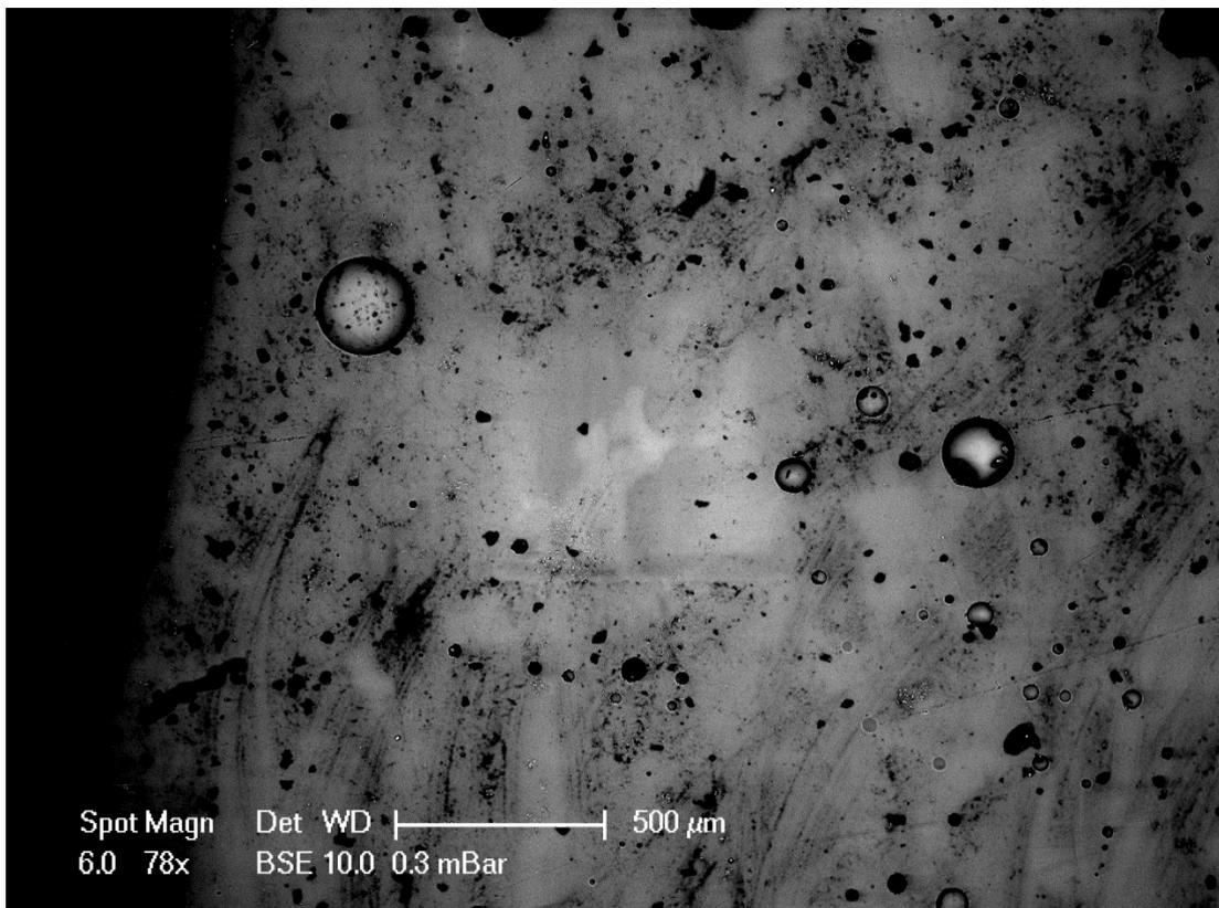
Figure 13: A close up image of FE brighter patch in one of the glasses, taken in CL on the SEM, EMMAC – University of Edinburgh.
