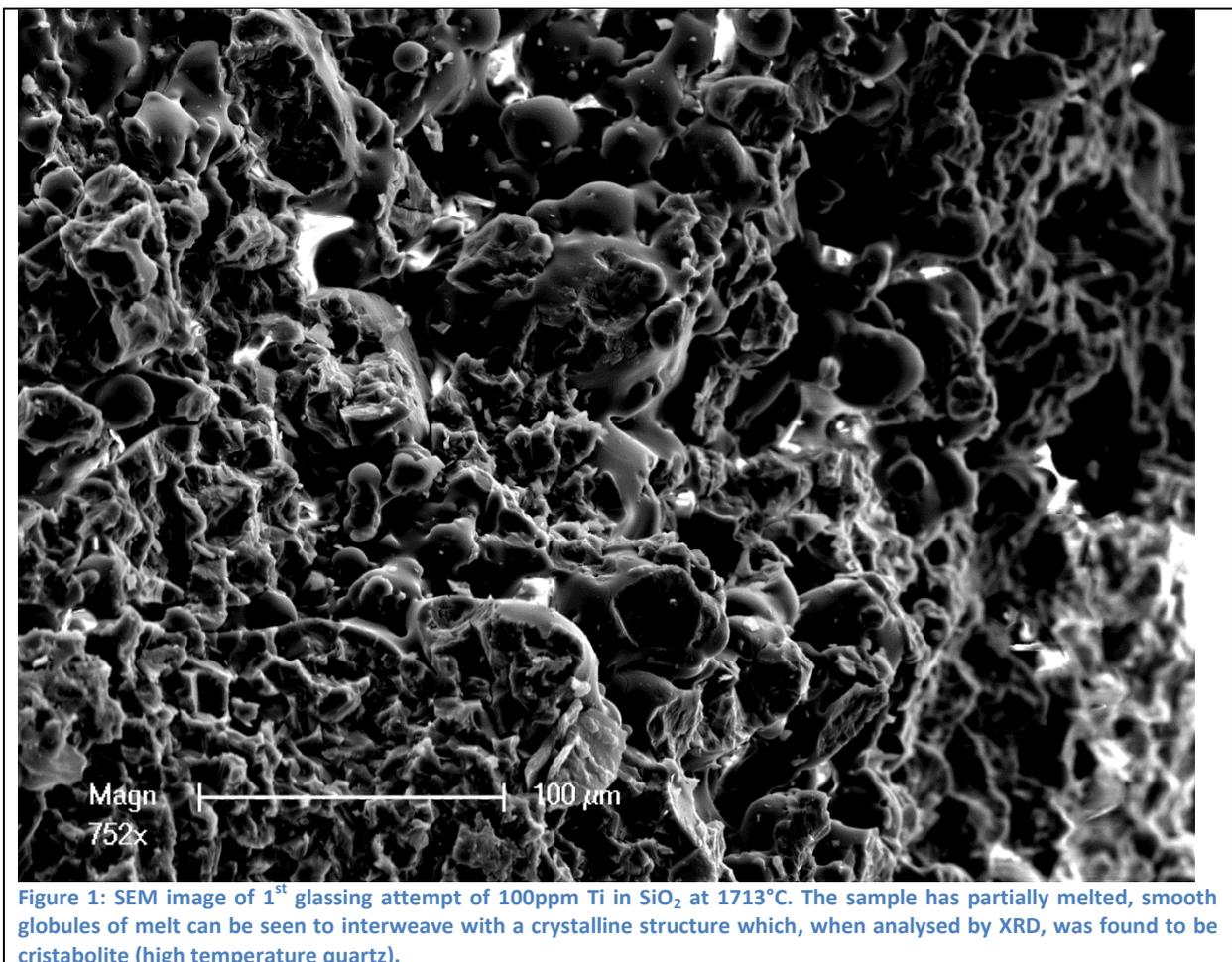
Figure 1: SEM image of 1<sup>st</sup> glassing attempt of 100ppm Ti in SiO<sub>2</sub> at 1713°C. The sample has partially melted, smooth globules of melt can be seen to interweave with a crystalline structure which, when analysed by XRD, was found to be cristobalite (high temperature quartz).
