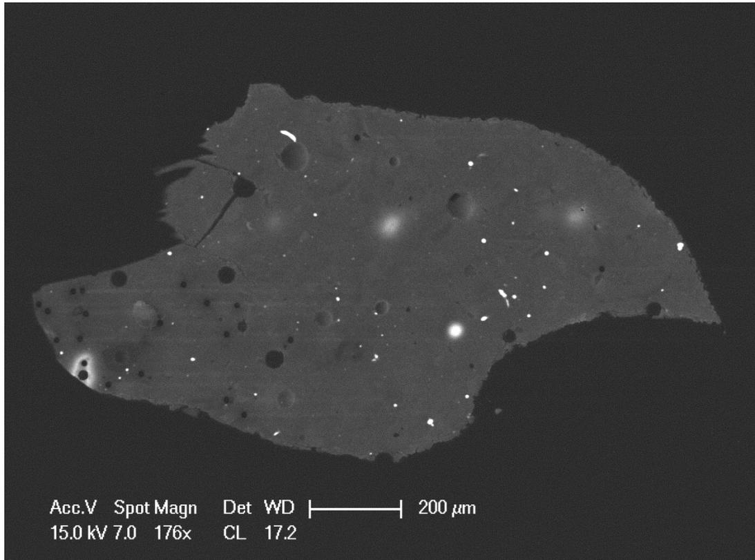
Figure 10: An image of Quartz glass 11 taken in CL on the SEM , EMMAC – University of Edinburgh. The lighter flecks are Fe, and not Ti that hasn't homogenised throughout the gel.
