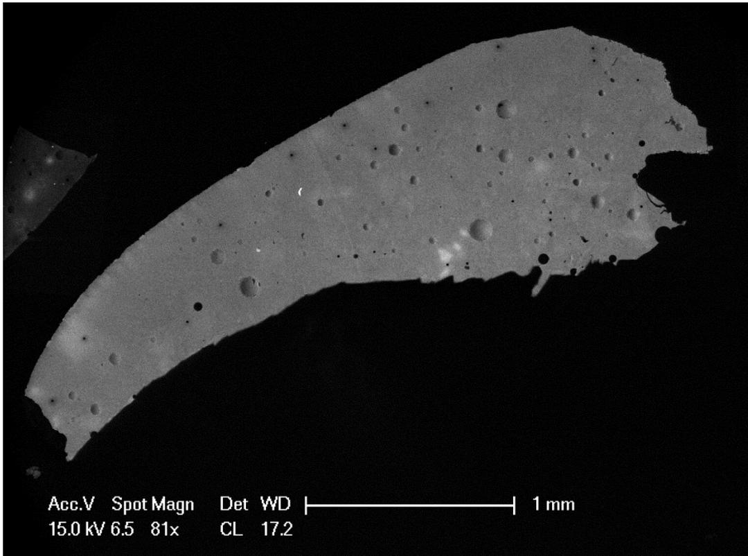
Figure 6: An image of Quartz glass 5 taken in CL on the SEM , EMMAC – University of Edinburgh. The lighter flecks are Fe, and not Ti that hasn't homogenised throughout the gel.
