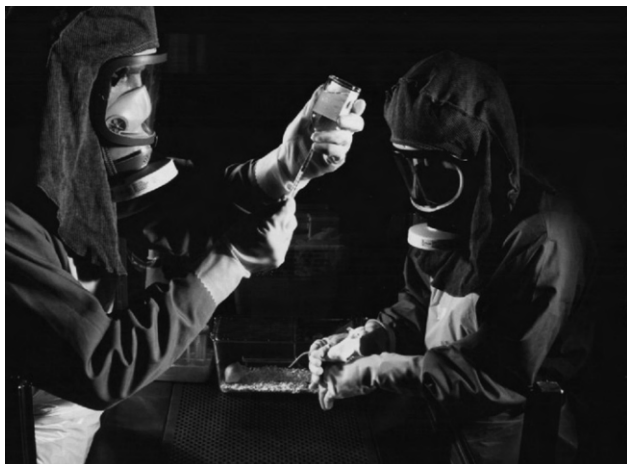
Figure 11.1 The use of RPE plus down-draught table to protect the operators during procedures on infected animals. (Courtesy of Health Protection Agency.)
