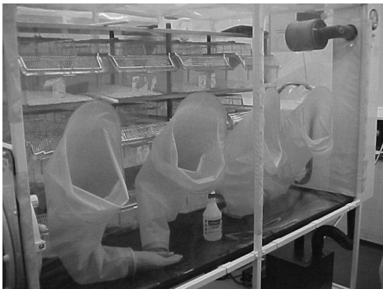
Figure 11.4 A flexible film isolator used to house infected mice or guinea pigs. (Courtesy of Health Protection Agency.)
