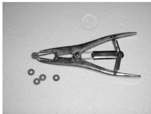
Figure 49.1 Elastic castration rings and applicator, an easy way of sealing fish transport bags.
