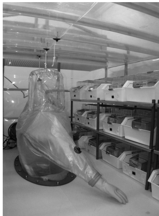
Figure 11.5 The interior of a half-suit isolator used to house infected guinea pigs. (Courtesy of Health Protection Agency.)
