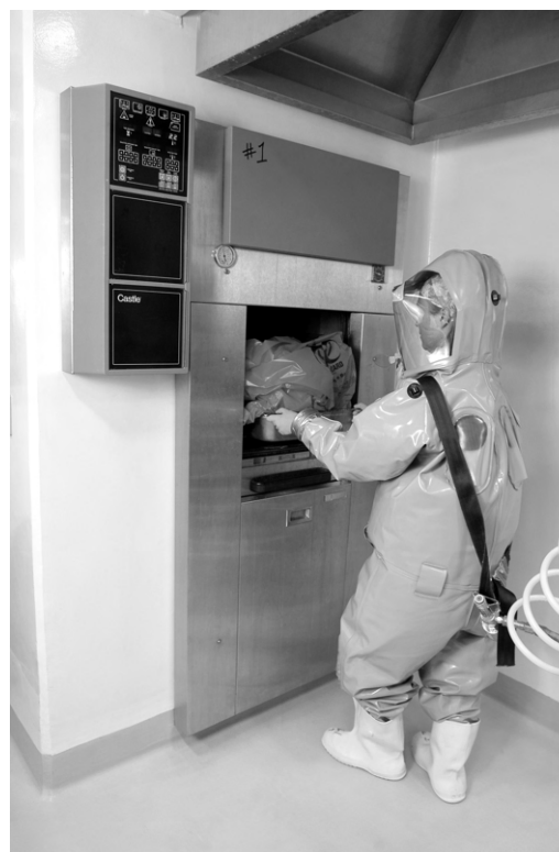
Figure 11.3 A one-piece full suit that might be required for work with dangerous pathogens. (Courtesy of the Canadian Science Centre for Human & Animal Health.)
