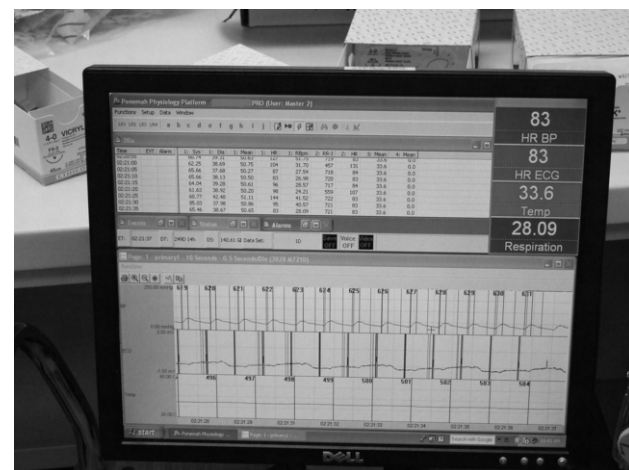
Figure 11.16 Real-time display of cardiac and respiratory data from a telemetry implant. (Courtesy of Health Protection Agency.)
