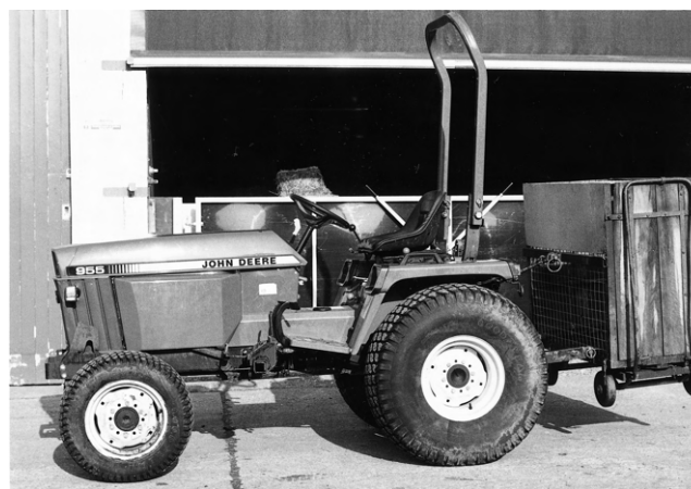
Figure 34.3 A home-made crate suitable for transporting one or two sheep or goats. Notice the couplings to allow carriage by tractor, plus the wheels and handle for manual pulling. Both ends can be lowered to form a stepped ramp, and the top can be lifted to access the animal.
