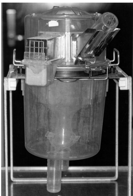
Figure 21.21 Metabolism cage with food hopper, water bottle and funnel. (Photo: T.P. Rooymans.)
