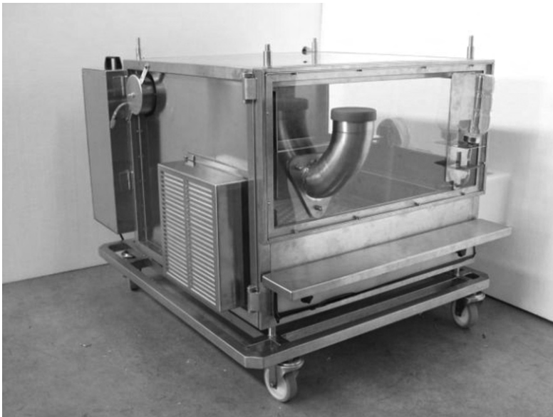
Figure 11.14 A ventilated unit for use with ferrets infected with a high-level pathogen. (Courtesy of Tecniplast UK.)
