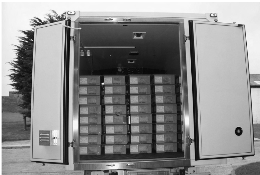
Figure 13.4 The back of a partially loaded, climate-controlled truck containing rodent shipping containers with integral ventilation stand-offs. The air channels between the containers allow circulation of air across the filtered openings.
