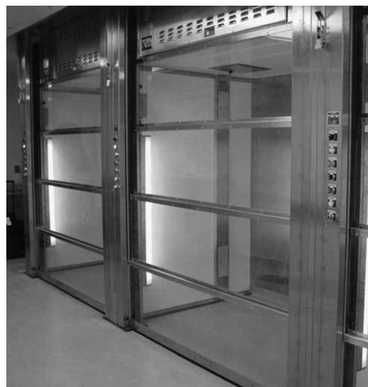
Figure 11.10 A typical containment booth with upwardly telescoping sectioned doors. (Courtesy of Britz & Co., USA.)
