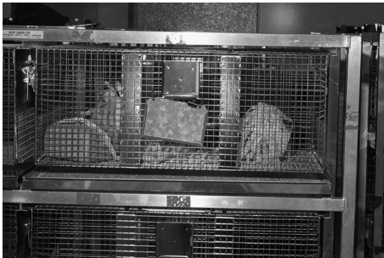
Figure 18.3 Wild rat cage showing the vertical runners down which metal partitions can be slid. Courtesy of The Food and Environment Research Agency, British Crown Copyright, 2009.
