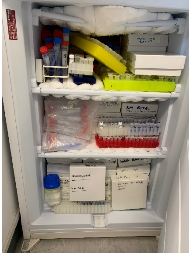
Figure 18. Icing reducing freezer space, access to contents is impeded and there is potential for damage to the unit (see top bar bent by the ice buildup). The absence of drawers also facilitates ice buildup.
