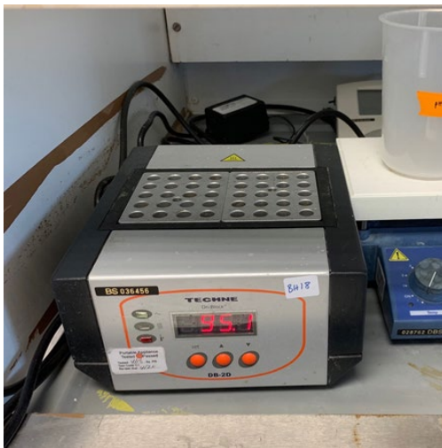
Figure 41. Block heater set to 95C, empty.
