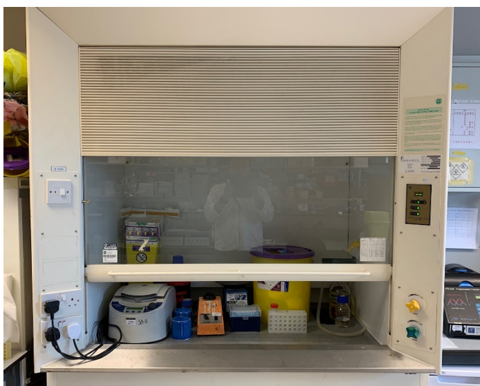
Figure 34. Fume cupboard where the sash has been left open with poor front and contents loading.
