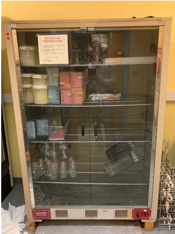
Figure 37. Old technology, 1000L drying cabinet.
