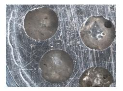
Reflected light photo-micrograph of four cored samples pressed into indium ready for gold coating and analysis.
