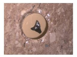
In this example a small fragment of BIR glass standard has been placed on to the brown tape. There has been slight fracturing of the back of the glass substrate.
