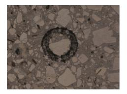
The crystal to be removed has been marked using the Nikon marker. The internal diameter of the ink-ring is ~2mm and easily visible to accurately align the drill bit to the required position.
