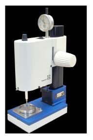
An ultrasonic disk drill is a proven method for producing thin disc shaped specimens from hard, brittle materials such as ceramics, glasses, polished thin sections, and geological materials. This technique produces disks (ID of ~1-3 mm) or cylindrical rods from bulk samples, or cut small diameter holes in thin sections free from significant edge and surface damage.
