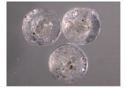
Three samples extracted from three separate polished thin sections. Each core is  $\sim 2mm$  in diameter with the area of interest in the centre. In this example, the olivine crystals contain rare melt inclusions and are being prepared for  $\delta^{11}$ B isotopic analysis.
