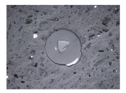
Reflected light photo-micrograph of the polished standard (BIR) and the surrounding thin section.
