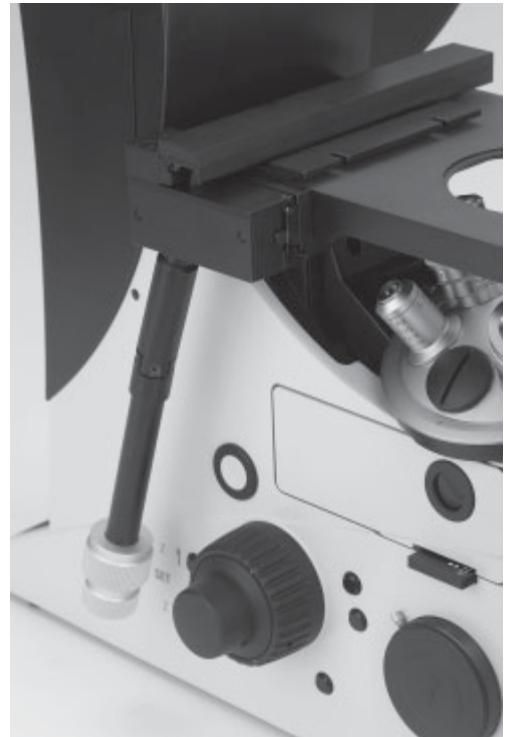
Fig. 25 Installation of attachable mechanical stage
