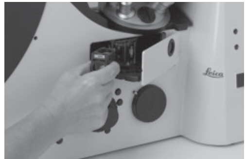
Fig. 68 Inserting or removing a filter cube
