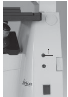
Fig. 92 Adjusting the field diaphragm (incident light-fluorescence)
