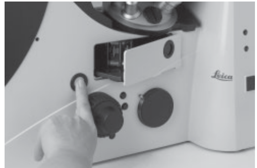
Fig. 68 Inserting or removing a filter cube
