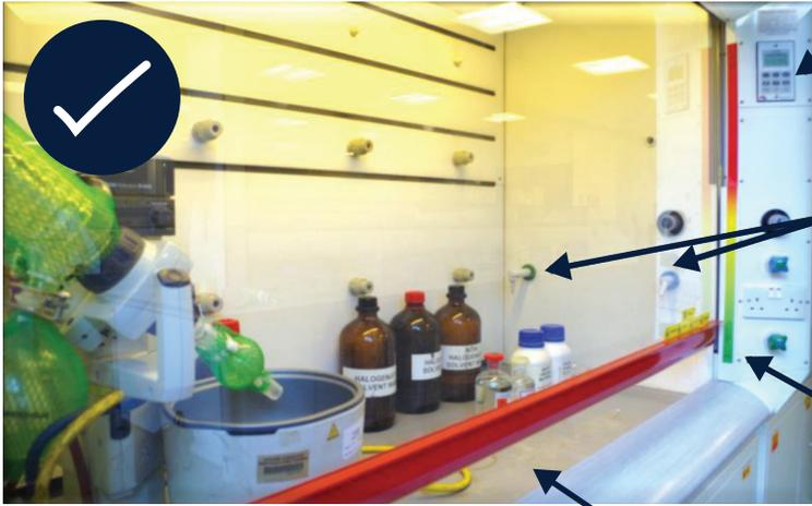
Check the fume cupboard is operating within the correct parameters.
