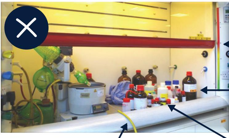
Sash is kept open above the yellow traffic light signal. This is a major health and safety risk and also increases the amount of energy used to maintain appropriate air flow.
