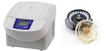
Centrifuge spins tubes at 14,000 revolutions per minute (rpm) for 2 minutes
