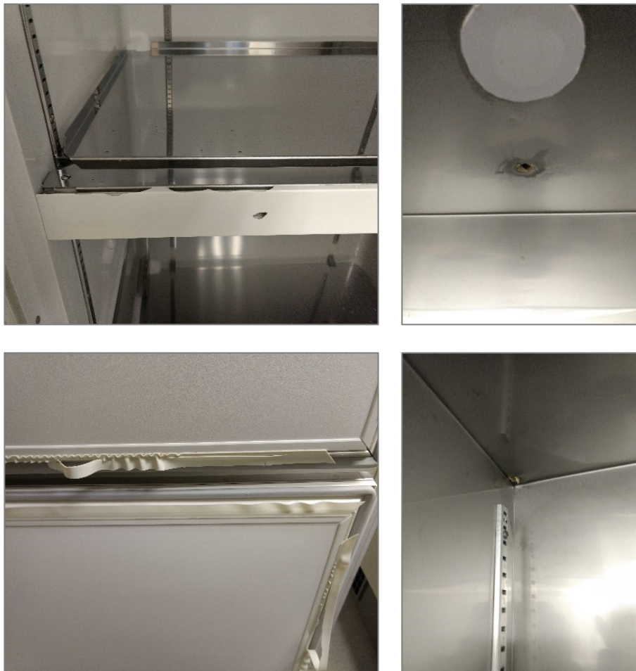
Figure 2. Examples of poor maintenance in freezers
