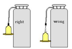
• Do not bend the dispensing pipe unnecessarily - Doing so may cause damage that will eventually cause the pipe to break;
