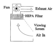
Figure 1: Schematic diagram of a Class I Microbiological Safety Cabinet
