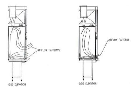
Figure 2: Schematic diagram of a Fume Hood (a. Sash open; b. Sash closed)
