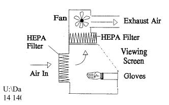
Some hybrid Class I/III cabinets exist, whereby a removable port may be attached to the front aperture of the cabinet. However, the construction and testing of these cabinets is such that when used in Class III mode it is *not* equivalent to the specification of a standard Class III cabinet.
