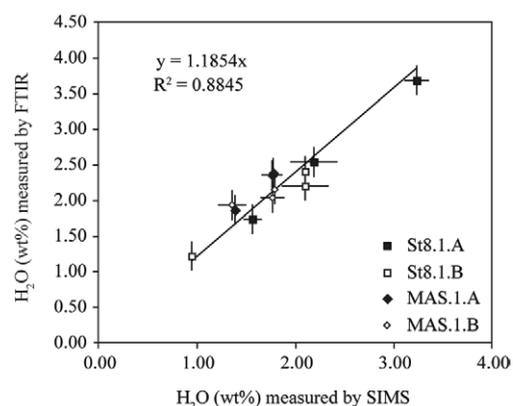
**Figure 4.** Comparison of H<sub>2</sub>O contents of experimental glasses measured by both FTIR and SIMS. Deviation from a 1:1 line is attributed to uncertainty in the extinction coefficient used for processing FTIR data. A correction factor of 1.1854 has been applied to all of the FTIR data to bring them into line with SIMS. No such correction was required for CO<sub>2</sub> data.
