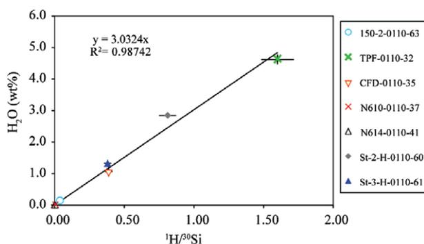
**Figure 1.** Working curve calibrated for basaltic melts using <sup>1</sup>H/<sup>30</sup>Si ratios of seven basaltic glass standards.
