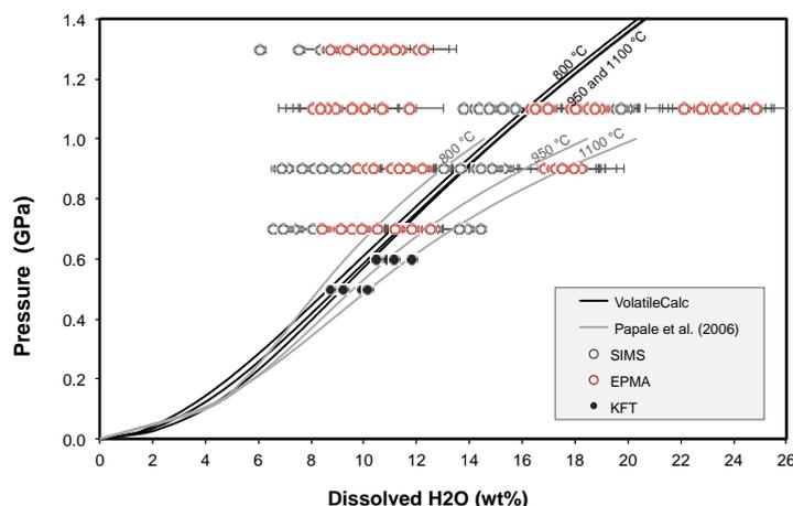
**Figure 1.** Pressure versus H<sub>2</sub>O content of glasses from solubility experiments, measured by SIMS, EPMA, and KFT. Water contents have been corrected for quench vesiculation using an appropriate equation of state, assuming a pure water vapour. Modelled H<sub>2</sub>O solubility curves from [3] and [4] are shown for reference.
