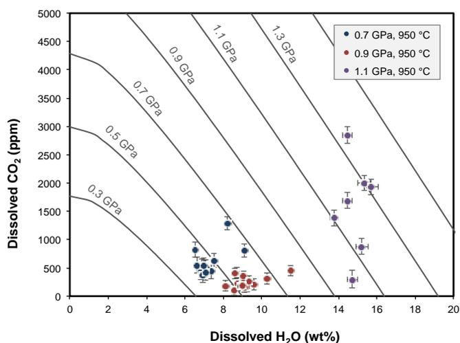
**Figure 2.** H<sub>2</sub>O and CO<sub>2</sub> contents of three experimental glasses measured by SIMS, plotted against modelled solubility isobars [3]. These runs were intended to be CO<sub>2</sub>-free, but carbon is clearly present. CO<sub>2</sub> contents inferred from carbon measurements are variable within each sample and range from hundreds to thousands of ppm.
