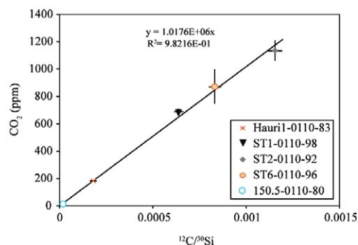
**Figure 2.** Working curve calibrated for basaltic melts using <sup>12</sup>C/<sup>30</sup>Si ratios of five basaltic glass standards.
