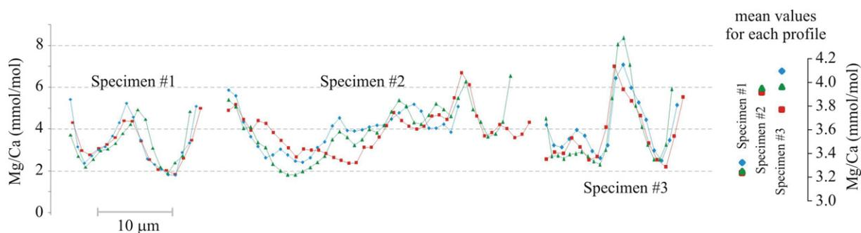
**Fig. 1** Reproducibility of Mg/Ca measurements of *G. sacculifer* final chambers using SIMS 1- $\mu\text{m}$  step profiling across the chamber cross-section. Three replicate profiles (marked by coloured symbols) show reproducible Mg/Ca patterns and average Mg/Ca values for each specimen (indicated on the right).
