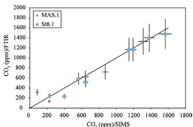
**Figure 3.** Comparison of CO<sub>2</sub> contents of experimental glasses measured by both FTIR and SIMS. Deviation from a 1:1 line is attributed to uncertainty in the extinction coefficient used for processing FTIR data.
