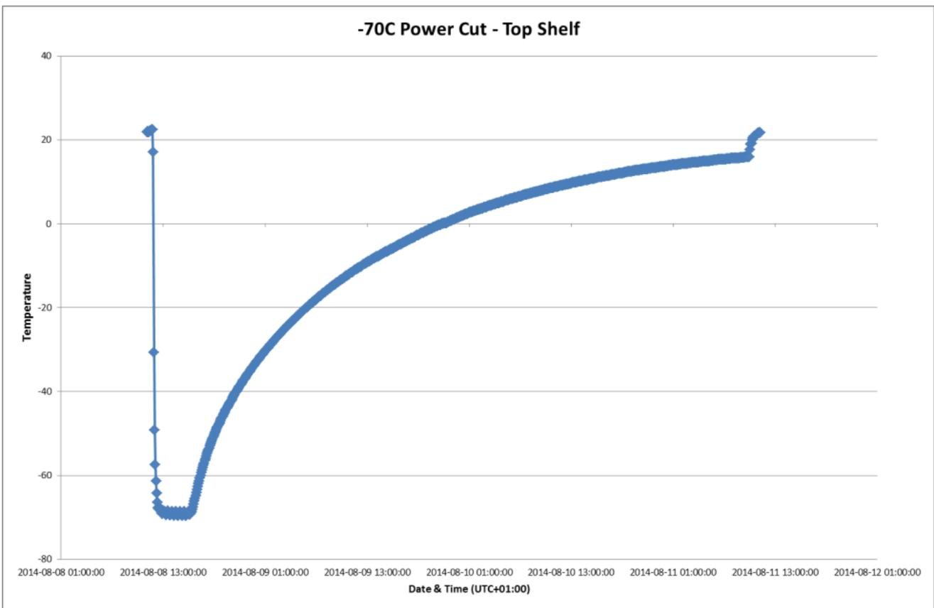
Graph 2: Typical temperature rise profile from power cut study. Note this is for a -70 °C freezer and the top shelf.
