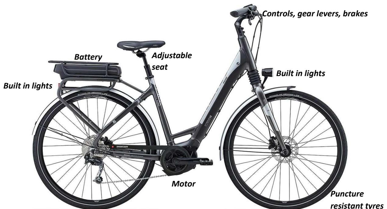
**Type of bike:** Giant Prime E+2 2015 - Electrically Assisted Pedal Cycle (EAPC)
